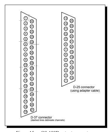
Figure 15 --- QS-100D output connectors
